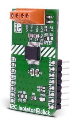
**12C Isolator 2 click** provides I2C lines and power isolation for slave devices. It carries the ADM3260 dual I2C isolator with an integrated DC-to-DC converter. I2C Isolator 2 click is designed to run on either 3.3V or 5V power supply. The click communicates with the target microcontroller over an I2C interface with additional functionality provided by the PWM pin on the mikroBUS™ line.
