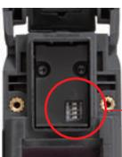
The mode of Operating Range Selection can be selected with the DIP Switches\* on the emitter.
