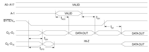
Notes: 1. Timing measurement references are 0.8V and 2.0V. Input AC drive levels are 0.45V and 2.4V, unless otherwise specified.
