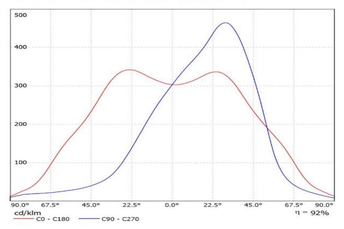
Luminaire: Ledil Oy CA11890\_Strada-SQ-T-DN-XM-L-TAPE CA11890\_Strada-SQ-T-DN-XM-L-TAPE Lamps: 1 x Cree XM-L(White)
