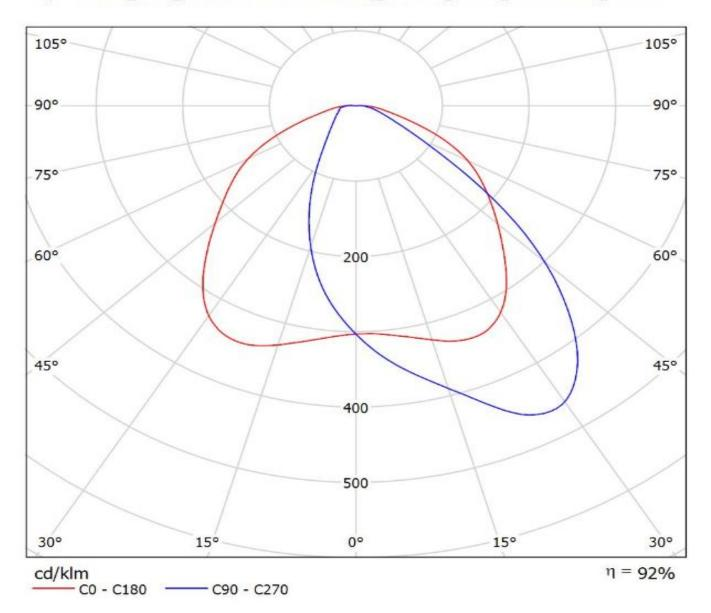
NOTE: The typical divergence will be changed by different color, chip size and chip position tolerance. The typical total divergence is the full angle measured where the luminous intensity is half of the peak value.
