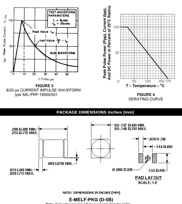
**Note:** If mounting requires adhesive separate from the solder, an additional 0.080 inch diameter contact may be placed in the center between the pads as an optional spot for cement as shown in the pad layout.
